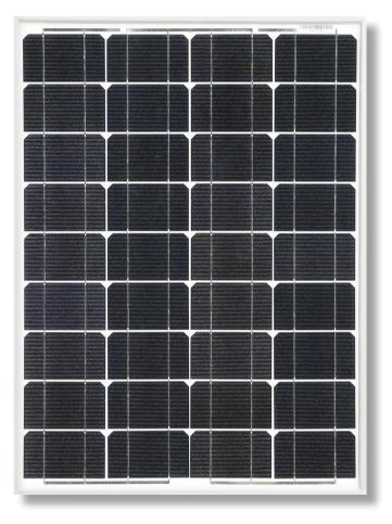
**HES solar modules** with high efficiency crystalline solar cells, offers high charge current at a voltage suitable for both summer and winter temperatures. The cells are bonded to a special tempered solar glass for watertight integrity and a deep anodized aluminum frame makes them strong and rugged for all Canadian environments.
