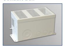
The ME-CB conduit box is designed to work with Magnum ME, MS, and RD Series Inverter/Chargers. It provides an enclosure for AC and/or DC wiring and has knockouts for ½", ¾", 1", and 2" trade-size conduit. The ME-CB adds just over 5" (13 cm) to the length of the inverter.
