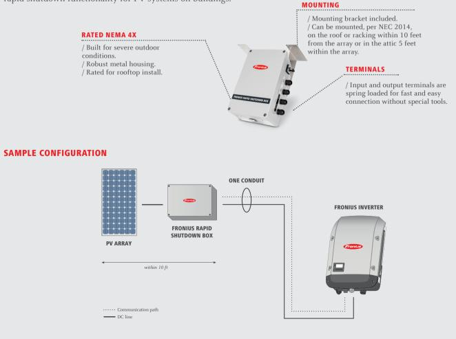
\* Excluding the Fronius Symo 15.0 -3 208 / Fronius Galvo only works with Fronius Rapid Shutdown Box Single
